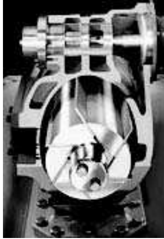
Figure 3.8 Cutaway view of a rotary vane compressor ( Courtesy of Pneumofore SpA ).
