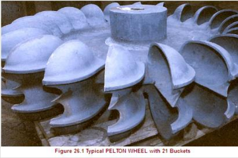
Figure 26.1 Typical PELTON WHEEL with 21 Buckets
